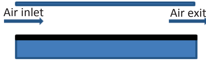
Figure 1. Schematic view of single duct solar collector.
